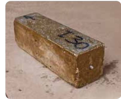
MAGNESIUM CHLORIDE after 168 Freeze / Thaw cycles in 15% \text{MgCl}_2 solution
