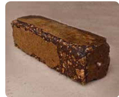
CALCIUM CHLORIDE after 168 Freeze / Thaw cycles in 17% \text{CaCl}_2 solution
