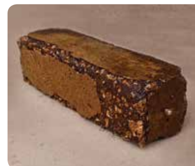
CALCIUM CHLORIDE after 168 Freeze / Thaw cycles in 17% \text{CaCl}_2 solution
