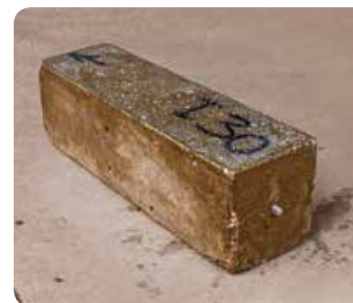
MAGNESIUM CHLORIDE after 168 Freeze / Thaw cycles in 15% \text{MgCl}_2 solution
